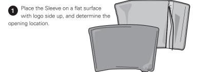
Be sure the Heat Exchanger is flat inside the Sleeve with no folds or creases. Zip up the Sleeve, if applicable. After assembly, lay the blue side up and ensure the Heat Exchanger is uniformly laid out and smooth inside the Sleeve.
