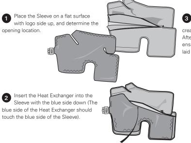
Be sure the Heat Exchanger is flat inside the Sleeve with no folds or creases. Zip up the Sleeve, if applicable. After assembly, lay the blue side up and ensure the Heat Exchanger is uniformly laid out and smooth inside the Sleeve.
